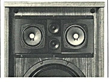
2-INCH CONE TWEETERS: A pair of 2-inch cone tweeters, vertically arranged, are charged with handling frequencies over 6.500Hz. The upper one is tilted to the left 3 degrees and the lower to the right by 3 degrees, resulting in improved sound dispersion and reinforced sound field effect. Each tweeter includes a very light vibrating system and reproduces treble notes of very clear, refreshing timbre. There is a very smooth transition to the midranges.
